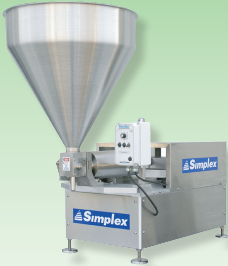
Simplex Model VS-1 with single straight spout, product cylinder and 10 gallon hopper
